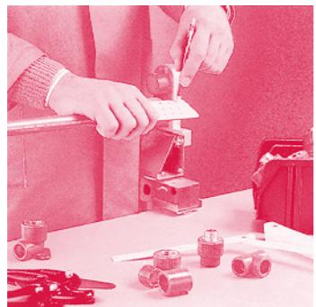
The welding depth is marked with a gauge and suitable marker
